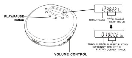
NOTE: The ESP PLUS™ function will turn on automatically when the PLAY/PAUSE button is pressed.
